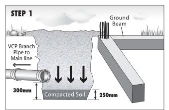
**STEP 1:** Locate position of chamber, dig hole to a depth of 300mm (1 foot) below the main sewer pipe connection. Backfill and level the bottom of the hole by tamping (compacting) the earth to 50mm below the socket of the outgoing pipe. For ground with High Water Table, anchor base of chamber to a concrete slab of width 600mm X 600mm and thickness of 100mm.
