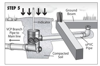
**STEP 5:** Place earth/concrete on the temporary cover holding an indicator pipe on top. Backfill the trenches and hole where the chamber is located tamping every 100mm of backfill being filled. Tamp to 100mm above the pipes and backfill to ground level where only the indicator pipes are visible to be able to locate the chamber in the future.
