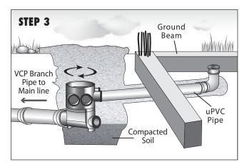
**STEP 3:** Locate the position of where all the pipes going to the Inspection Chamber will enter the ground level. Dig trenches sufficiently wide and depth of the trench should be sufficient to allow the pipes to pass below the ground beam. Rotate the Body of the Chamber such that the maximum numbers of sockets are able to be fixed to the incoming trenches. Trenches that are not in line with the sockets of the Inspection Chamber can be joined to the Chamber by the use of 45° bends.
