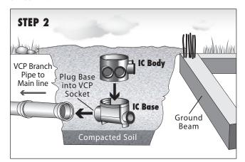
**STEP 2:** Connect the base of the inspection chamber to the pipe leading to the main sewer line, if there is no existing pipe, connection can be done in the future. Rotate body to the best suitable position and push fit into base. Use liquid level gauge to ensure the inspection chamber is level.
